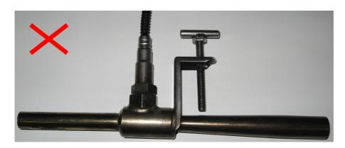
Inaccurate, poorly designed probe (too small & fixed clamp position)!
